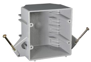
EZ32DNZ EZ BOX is a 32 cu. in., 2-gang, electrical switch and outlet box for residential or light commercial electrical installations. It features screw-nails for use on aluminum, light to medium grade steel or wood studs. The sharp point, slotted head and threaded body allow for easy installation using a power screwdriver without having to predrill. It can also be installed on wood studs using a hammer.
