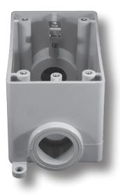
Exposed Boxes Type FDC designed for use in indoor and outdoor locations where boxes are exposed and subject to environmental conditions. Type FDC is intended for straight line conduit runs with one opening on each of the two short walls of the box. FD boxes are the deepest exposed boxes. They provide space for large devices and additional wiring capacity.
