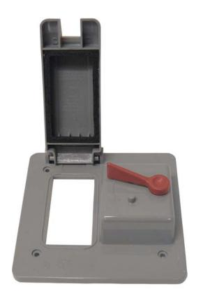
Weatherproof when closed. Fits a two gang FS type box. Toggle operates a double or single pole 115 volt switch. GFI opening fits a ground fault interrupter receptacle. For outdoor service.
